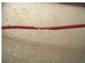
Soldering, Note: joint self-supporting
