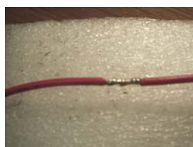
Use shank of iron to shrink sleeve by gently smoothing over surface.
